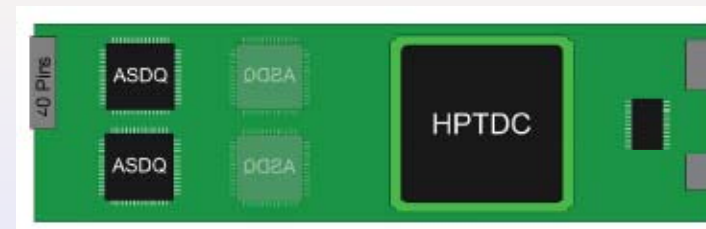
2 ASDQ + TDC on a board
